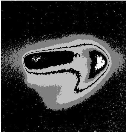
Fig. 4. Image obtained by scanning a photograph obtained in 190 mTorr oxygen, for a delay of 600 ns from the impact of the laser pulse onto the target. Weak emission is visible in front of the luminous plasma front, at its tip. The white regions are the most luminous, followed by the compact black ones around them.
